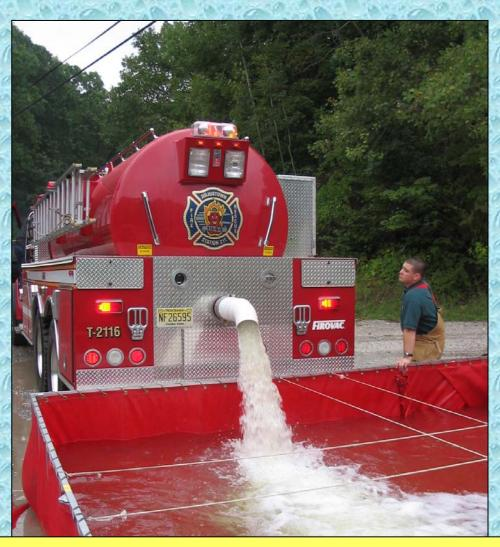
When the vacuum pump is engaged (in the reverse mode) the tank is pressurized and the water is forced out in an impressively short amount of time.
