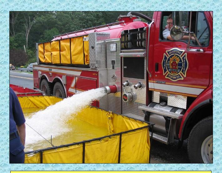
With the tank pressurized – water is blown out of the tank!
