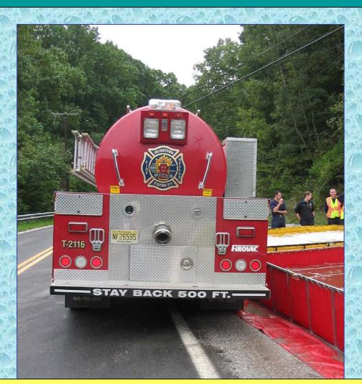
However, for loading and off-loading, the rig uses its highvolume vacuum pump. This photo shows the tanker's rear dump.
