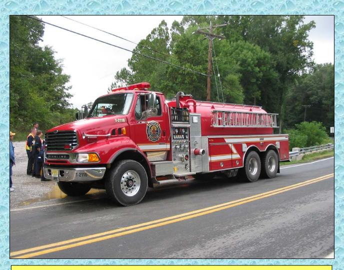
This 3000-gallon vacuum tanker was designed and built by Firovac, an Ohio company that specializes in vacuum tankers for fire departments.
