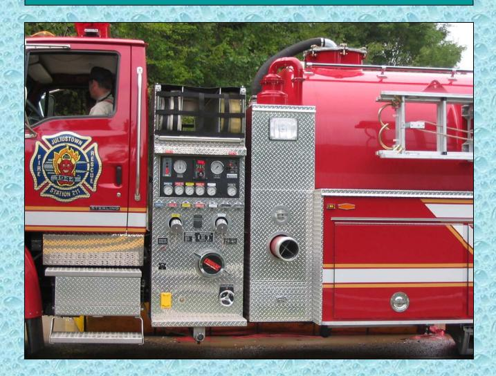
If needed, the rig is equipped with a centrifugal fire pump should it find itself having to pump to another pumper or having to pump an attack line.
