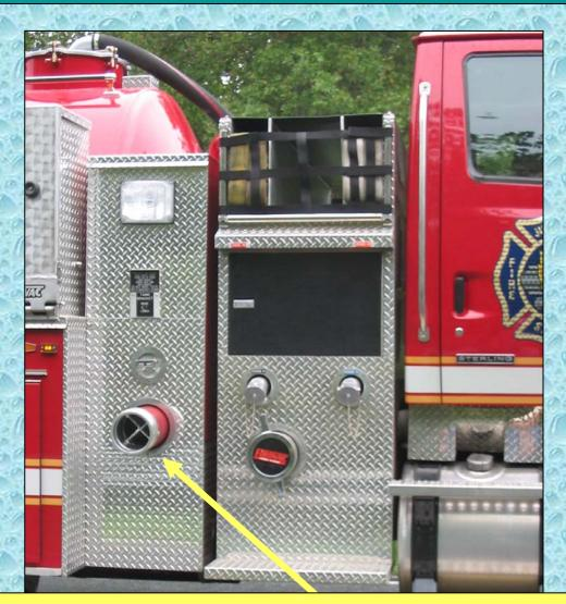
The tanker also is equipped with side dumps – one on each side of the rig.
