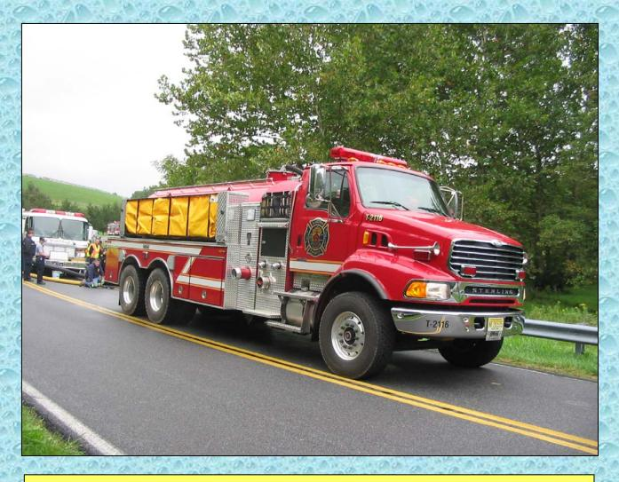
The tanker is equipped with two, 3,500 gallon dump tanks – one for the dump site and one for the fill site (if needed).
