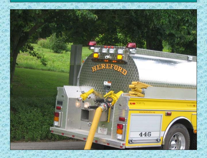
The 2005 tanker is also equipped with a large, direct-fill line which allows for quick refilling operations.
