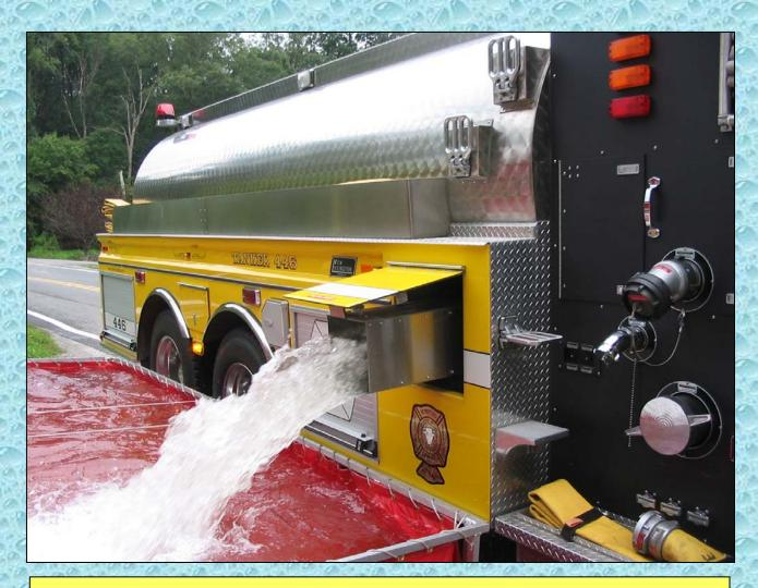
This dump chute is controlled remotely from the cab so that driver never has to leave the rig – which is ideal for reducing dump time.
