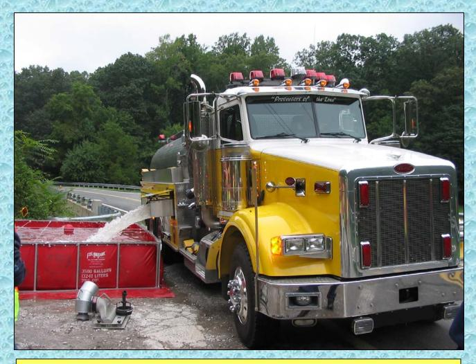
Shown here in action at the South Carroll Water Supply Shuttle, Tanker 446 uses one of its 10-inch side dumps to quickly off-load its water.
