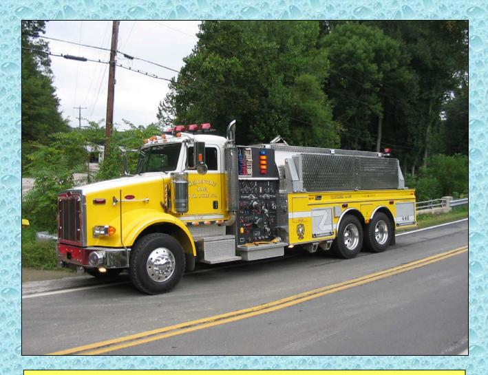
This 3000-gallon tanker is a "big water" hauler that is setup very nicely for delivering water in any rural water supply operation.
