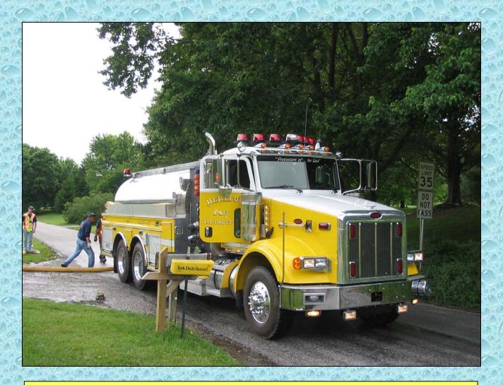
The elliptical tank shape allows for a lower profile which provides for a more stable drive and a lower center of gravity.
