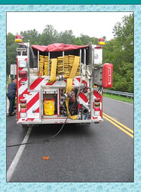
The rig carries 2,000 ft of 4-inch supply hose making it a versatile piece in non-hydranted areas.
