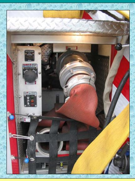
This rear intake is equipped with a master intake valve and is designed to provide full-flow for both drafting and hydrant system operations.
