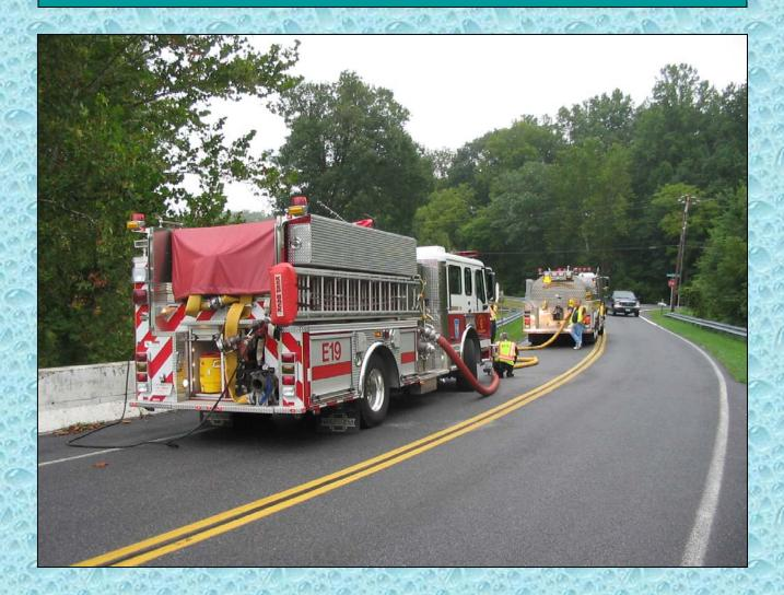
Shown in action here at a water supply drill, this 1250 gpm pumper operates as the fill site engine using LDH to support tanker fill operations.
