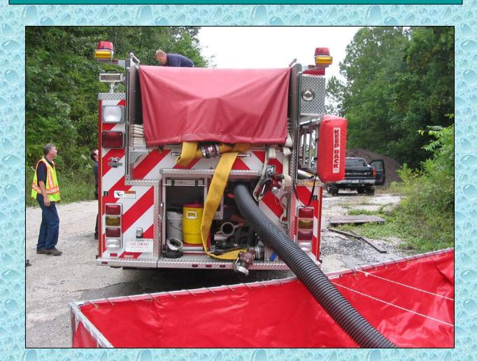
The rear intake in use at a dump site operation. The use of the rear intake allows for better positioning on narrow roads and driveways.
