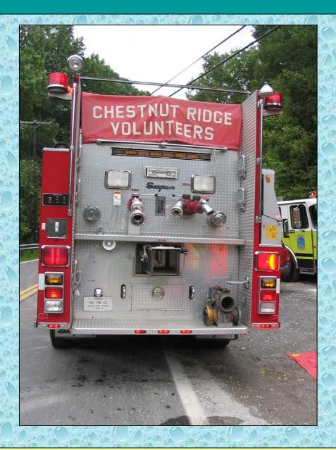
Engine Tanker 503 is equipped with a 1,750 gpm, single-stage Hale Q-Max pump and carries 1,200 ft of 5-inch LDH.
