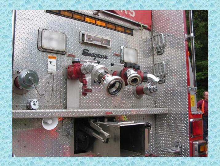
The rear end of this engine tanker is outfitted to intake and discharge water in a number of ways. The most important – the 10-inch Newton dump for gravity off-loading.
