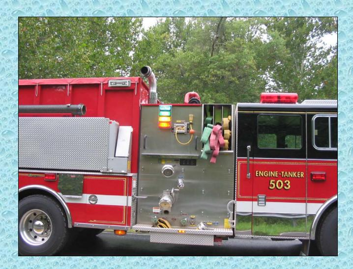
The rig is equipped with large, tank level indicator lights so that everyone can see the amount of water left in the 2,500 gallon on-board tank.
