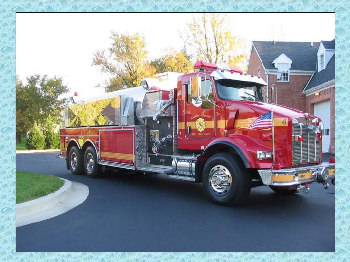
A 3,500-gallon dump tank is carried on the officer's side and is equipped with a powered lowering and raising lift.
