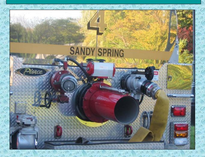
Besides this rigs side dump chutes, this rear chute can really off-load the water in a big way!
