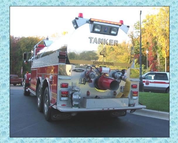
The elliptical shape of the tank allows for better handling on the road while still taking advantage of head pressure for gravity offloading..
