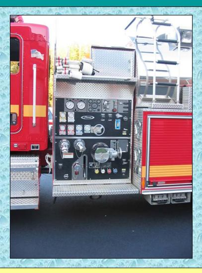
Tanker 704 is equipped with a 1,250 gpm, single-stage Waterous pump.
