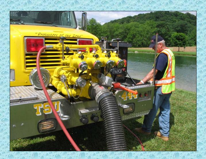
The 1000 gpm front mounted pump allows easy access to drafting sites.
