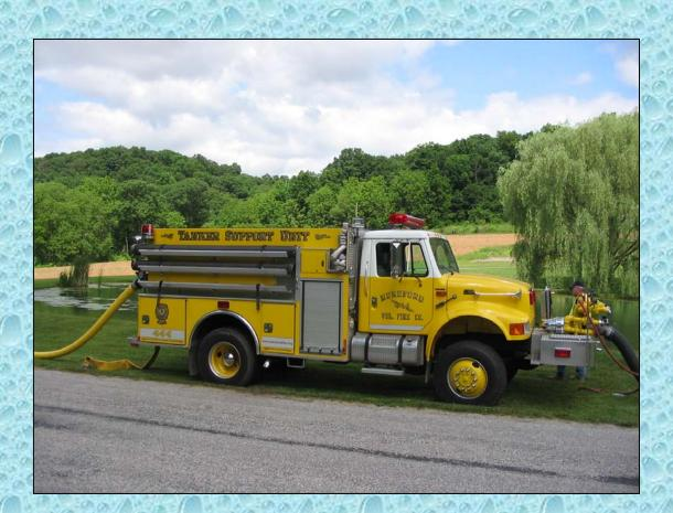
Operated by the Hereford VFC in Baltimore County, MD – this 1998 rig was built by New Lexington and was designed to support rural water supply and tanker operations.
