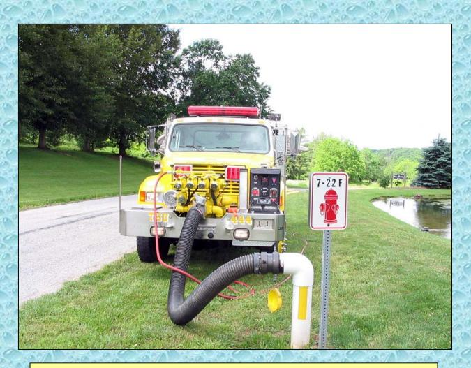
Shown in action here at the Route 30 Corridor water supply drill in June 2006. TSU 444 drafted from this dry hydrant in Pennsylvania and filled tankers hauling water back into Maryland.
