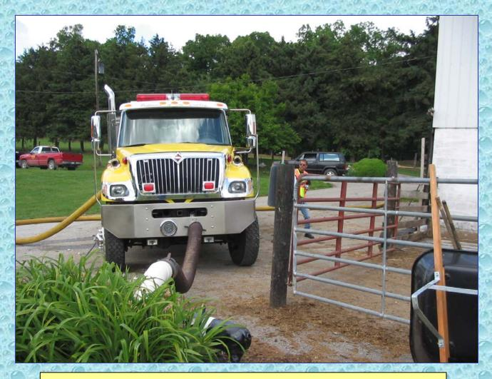
Shown in action here at a water supply drill, SU-6 takes suction from a DFH at a local farm pond and supplies a tanker fill manifold 800-feet away up a farm lane.
