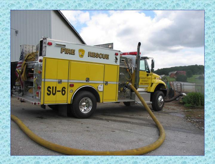
SU-6 has both a side-mounted and a rear-mounted high-flow discharge which can pump the rig's 1500 feet of 5-inch LDH.
