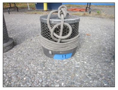
Figure 31: Akron Barrel Strainer Style 340. The strainer used a short, 8-inch diameter tube with approximately six hundred twenty-eight, 3/8-inch holes – some of which were in the closed end of the strainer. The holes all had sharp edges.
