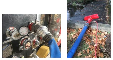
Figure 6: A 4-inch hose line supplied water to a Hose Monster flow diffuser with fixed-pitot. The hose line was 50 feet in length.
