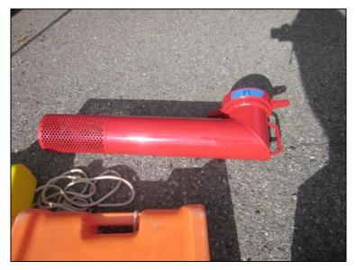
Figure 40: Kochek Ice Strainer (IS60). The strainer used 6-inch tubing and had approximately nine hundred fifty, 3/8-inch holes.
