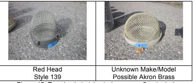
Figure 45: Two, basket-style strainers were flow tested.
