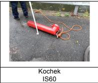
Figure 47: Only one ice strainer was flow tested.
