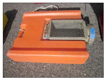
Figure 21: Fol-Da-Tank Float Dock floating strainer (FDS6). The strainer had a removable float that allows the strainer to be used as a box strainer. The strainer had approximately 90 square inches of open space in the expanded metal mesh.
