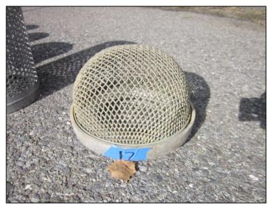
Figure 29: Basket Strainer (Unknown Manufacturer). The maker of this strainer was unknown, although the design resembles an Akron basket strainer. The strainer used ¼-inch wire mesh. Due to the design of the basket, there was limited uniformity in the mesh's hole size. The base of the screen had a 29-inch circumference.
