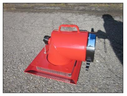
Figure 14: Kochek Big Water Low Level Strainer with 1.5-inch jet siphon (LL602). This strainer used an 8-inch tube.
