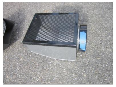
Figure 26: Kochek Box Strainer (BX60). The strainer used a welded-sheet metal housing and had approximately 114 square inches of open space in the expanded metal mesh screen.
