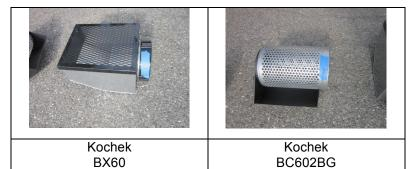
Figure 44: Two, box-style strainers were flow tested. The barrel strainer with bottom guard was used because it deploys and operates much like a box strainer.
