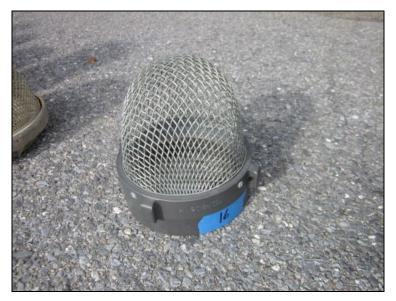
Figure 28: Red Head Style 139 Basket Strainer. The strainer used ¼-inch wire mesh. Due to the design of the basket, there was limited uniformity in the mesh's hole size. The base of the screen had a 22-1/4-inch circumference.
