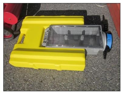
Figure 22: Ziamatic Floating Strainer (FDS-600-NST). The strainer had a removable float that allows the strainer to be used as a box strainer. The strainer had approximately 127 square inches of open space in the wire mesh.
