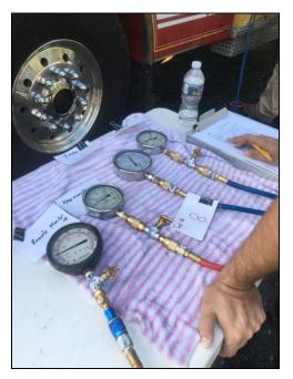
Figure 8: Each test gauge was connected remotely to a pressure measure point while the actual gauge was displayed on a central workstation table. This arrangement allowed for easy and efficient data collection.
