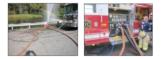
*Figure 5: Dual, 3-inch hose lines supplied water to a portable monitor. Each hose line was 50 feet in length.*
