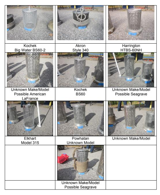
Figure 46: Ten, barrel strainers were flow tested.
