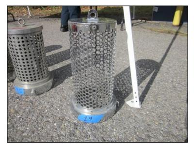
Figure 36: Elkhart Barrel Strainer (Model 315). The strainer had approximately seven hundred sixty, 7/16-inch holes. There were no holes in the end of the strainer. The holes all had smooth edges.
