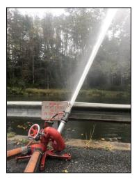
Figure 7: The Hose Monster was outfitted with a 2-1/2-inch orifice. The portable monitor was outfitted with an Akron flow test kit and 1-3/4-inch orifice.
