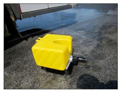
Figure 25: Task Force Tips Floating Low Level Strainer Jet Siphon (A03HNX-JET-F). This is the same strainer as used in the low level strainer flow test. The strainer had a cast housing; no tubing was used in the design.
