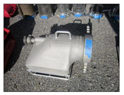
Figure 18: Firovac Low Level Strainer with 1.5-inch jet siphon (HVLL). The strainer had a cast housing; no tubing was used in the design.
