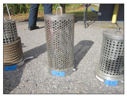
Figure 38: Barrel Strainer (Manufacturer and model unknown). The strainer had an outside diameter slightly greater than 7-inches and had approximately nine hundred sixty-eight, 5/16-inch holes. There were no holes on the end of the strainer. The holes all had sharp edges.
