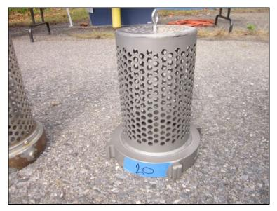
Figure 32: Harrington Barrel Strainer (HTBS-60NH). The strainer used 6-inch diameter tubing with approximately six hundred forty, 3/8-inch holes – some of which were in the end of the strainer. The holes all had sharp edges.
