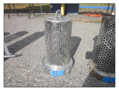
Figure 34: Kochek Barrel Strainer (BS60). The strainer used 6-inch tubing with approximately seven hundred ninety-eight, 3/8-inch holes. There were no holes in the end of the strainer. The holes all had sharp edges.
