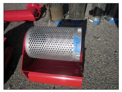
Figure 19: Kochek Big Water Self-Leveling Floating Strainer (FBS602). The strainer used an 8-inch barrel with more than one thousand, 3/8-inch holes.
