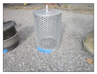
Figure 30: Kochek Big Water Barrel Strainer (BS60-2). The strainer used an 8-inch diameter tube with approximately twelve hundred sixteen, 5/16-inch holes – some of which were in the closed end of the strainer. The holes all had sharp edges.
