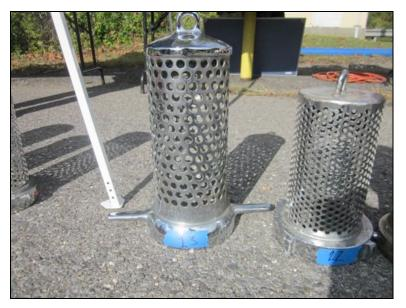
Figure 35: Barrel Strainer (Manufacturer and model unknown – possible Seagrave). The strainer came from a 1959 Seagrave pumper and had approximately three hundred sixty, ½-inch holes. There were no holes in the end of the strainer. The holes all had smooth edges.
