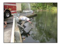
Figure 9: With the exception of the floating strainer tests, each strainer was deployed to a depth of 25-inches – meaning the top of the strainer was 25-inches below the surface of the water. A yardstick was used for measurement verification each time a strainer was deployed.
