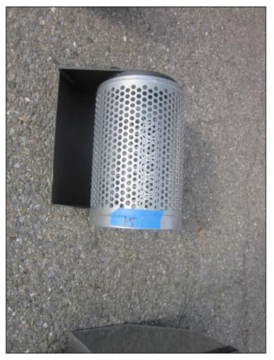
Figure 27: Kochek Big Water Barrel Bottom Guard Strainer (BS602BG). The strainer used an 8-inch barrel with more than one thousand 3/8-inch holes. This is the same barrel as was used on the Big Water Self-Leveling Strainer.
