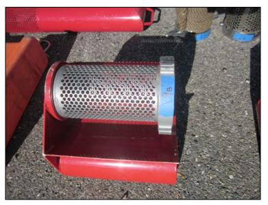
*Figure 20: Kochek Self-Leveling Floating Strainer (FBS60). The strainer used a 6-inch barrel with nine hundred and fifty, 3/8-inch holes.*
