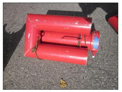
Figure 24: Kochek Floating Strainer (original model). The strainer used 6-inch tubing with approximately four hundred forty-four, ½-inch holes.
