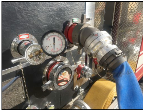
Figure 6: A 4-inch hose line supplied water to a Hose Monster flow diffuser with fixed-pitot. The hose line was 50 feet in length.
