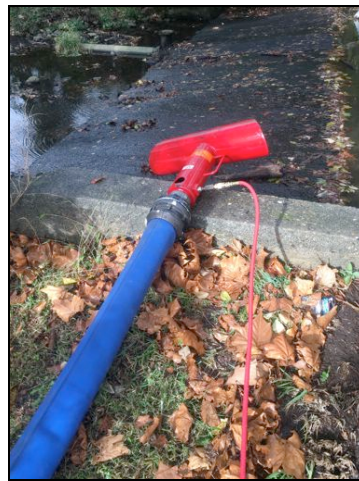
Figure 6: A 4-inch hose line supplied water to a Hose Monster flow diffuser with fixed-pitot. The hose line was 50 feet in length.
