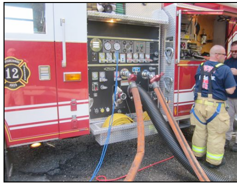
Figure 5: Dual, 3-inch hose lines supplied water to a portable monitor. Each hose line was 50 feet in length.
