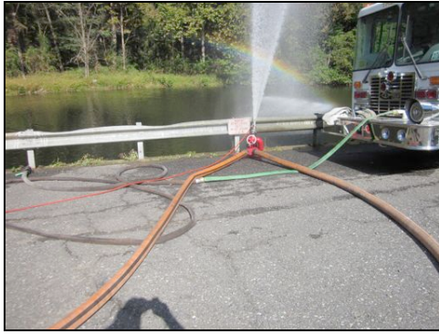
Figure 5: Dual, 3-inch hose lines supplied water to a portable monitor. Each hose line was 50 feet in length.
