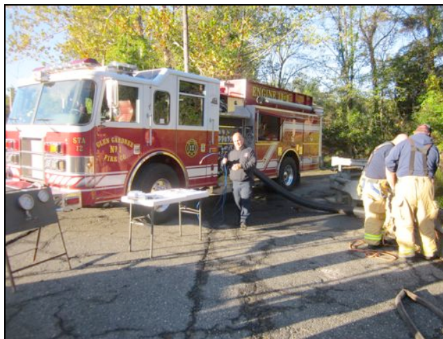
Figure 3: The Glen Gardner Fire Company supplied a pumper and crew for the project. Engine 1262 is a 2003 Pierce pumper outfitted with a 2,250 gpm Hale QMax pump and a 515 hp diesel motor.
