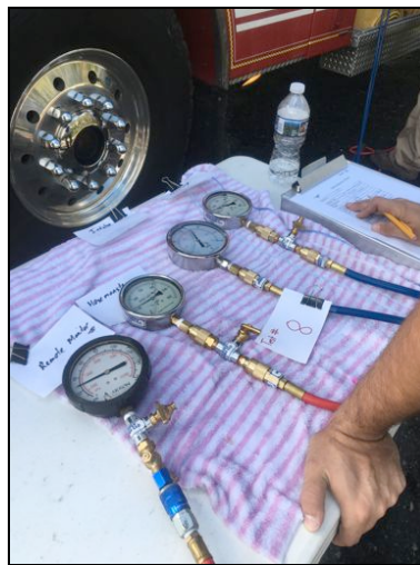
Figure 8: Each test gauge was connected remotely to a pressure measure point while the actual gauge was displayed on a central workstation table. This arrangement allowed for easy and efficient data collection.
